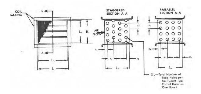
**4.1.2.2** Staggered tubes (as shown below) with smooth or crimped spiral fins or with flat plate or configurated plate fins on individually-finned tube. Air baffles shown are to be considered optional and *H* may be the distance between channels as shown in **4.1.2.1**.
